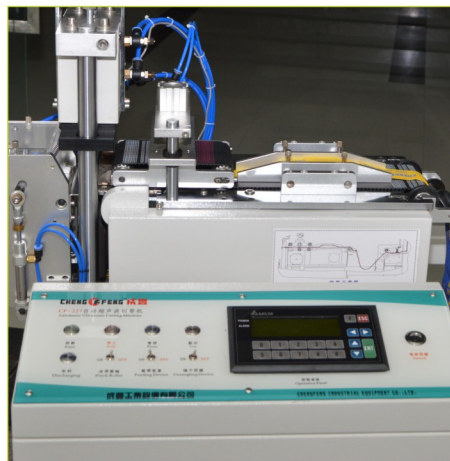
獨特的履帶式送料 Unique crawler type feeding structure
